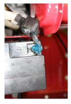
19. Screw live and neutral cables into place on battery (marked black and red on the battery).
