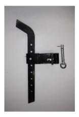
21. Place depth gauge into rear slot on machine. Adjust the pin for desired height.
