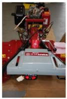
20.Screw in the tool box to the top of handlebars.
