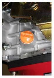
Gearbox oil – Using silver filler cap located on drive shaft, fill with oil. MAX 2.5 Litres Check levels using dip stick
