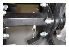
To fit the tines to the machine, remove the pins holding the wheels on. Remove the wheels, and slide on tines. Place red end caps on the ends and secure using the pin.
