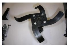
Repeat this to place all four tines around the bar. Bolt all four corners tightly.
