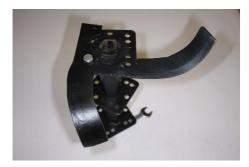
Lay one right handed tine onto tine bar, curling up. Then place a left handed tine across this one, curling down and bolt in the middle (left).
