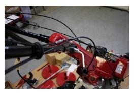
8. Remove adjustment bolt and lever (above left) and slide handlebars onto handrail stand. Replace bolt ensuring that the bolt goes into hexagonal hole (above middle). Tighten with lever to adjust to desired position.
